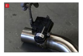
Once happy with fitment of Scorpion Exhaust, fully tighten up all clamps and fixing and plug in the electronic valve motors.
